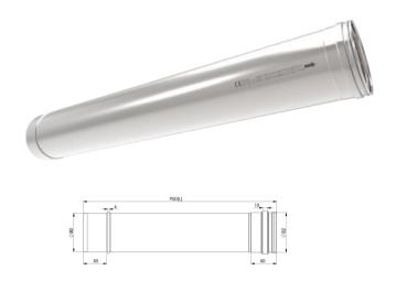
These are the main components of flues. They are generally produced at a length of 1000 mm. Straight modules are be made in different dimensions. Materials vary according to burner devices to be used with flues. 500mm and 250mm lengths are also made available to customers. They are produced in the range of Ø80mm to Ø1200mm.
