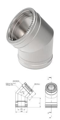
Elbows are used on horizontal and vertical lines. They are used for bypassing deviations on the route determined for flue assembly. It is produced with 45-30-15 degree angles. Its material grade is 304 or 316. 304 and 430 grade material can be used as coating sheet on double walled systems. Insulation thickness is 25 mm as standard. However, it is also produced with special dimensions.
