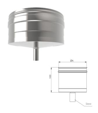
It is used for collection and transfer of condensate in flues. It is installed vertically below the inspection cover. It can be used horizontally on cascade systems. 304 and 430 grade material can be used as coating sheet on double walled systems. Insulation thickness is 25 mm as standard. However, it is also produced with special dimensions.
